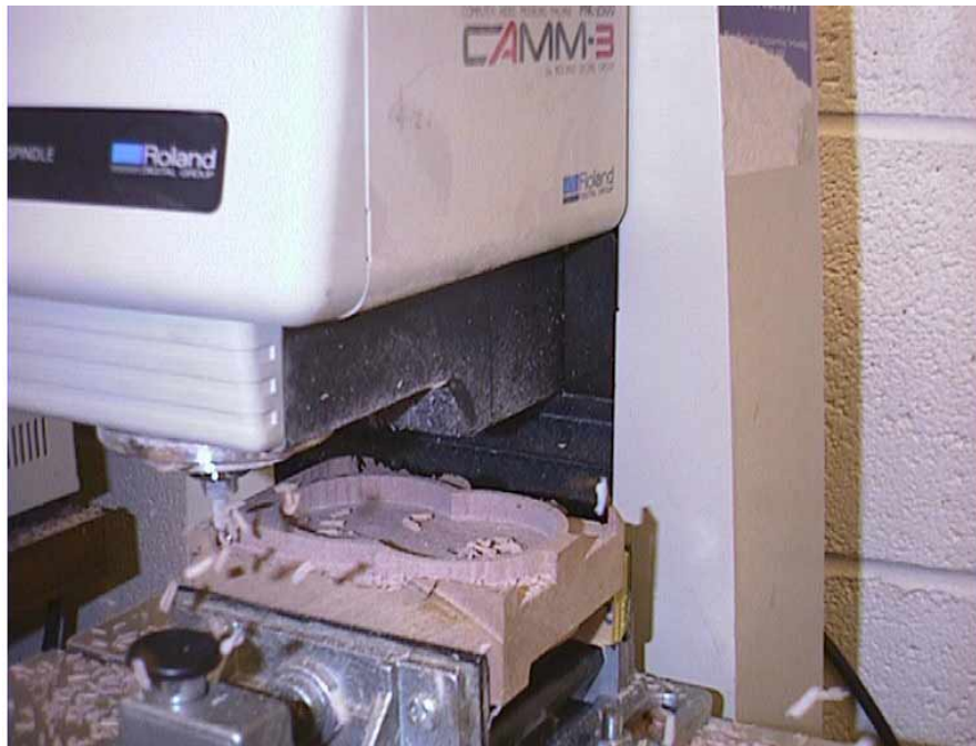
Fig. 8. Machining Case out of Plastic on the Roland Prototyping Mill
