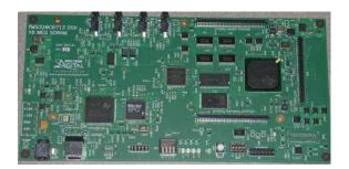
Figure 1. The TMS320C6713 DSK board.
