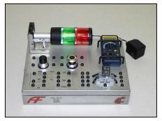
Laboratory 1: This laboratory emphasizes the most fundamental concepts of PLC ladder diagrams using fully hardware implemented control logic. This is the first time students are exposed to normally-open, normally-closed contact types, relays and ladder diagrams. Therefore, we designed and built custom pieces of hardware and mailed them to each remote site. This is the only experiment that does not require remote control and programming of hardware over the Internet. Students explore the contact
