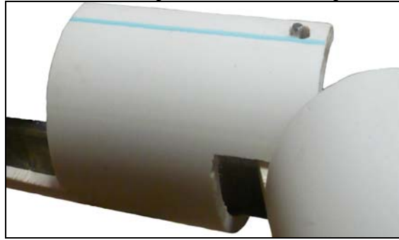
Figure 5: View of second phalanx showing rigid pieces
