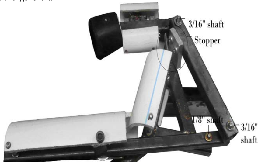
Figure 17: Improvements made on upper fingers
