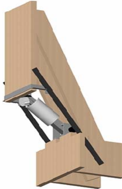
Figure 13: AutoCAD drawing of the thumb
