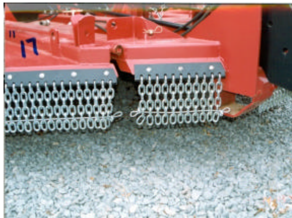
Figure 7 (C). Cable and Clamps Threaded on Both sides of the Mower's Guard
