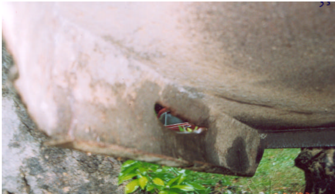
Figure 10. The Gash in the Mower Housing Where the Blade Exited
