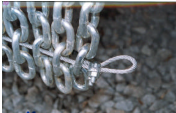
Figure 7 (b). A Wider View of Cable and Clamp Threaded on One Side of the Guard
