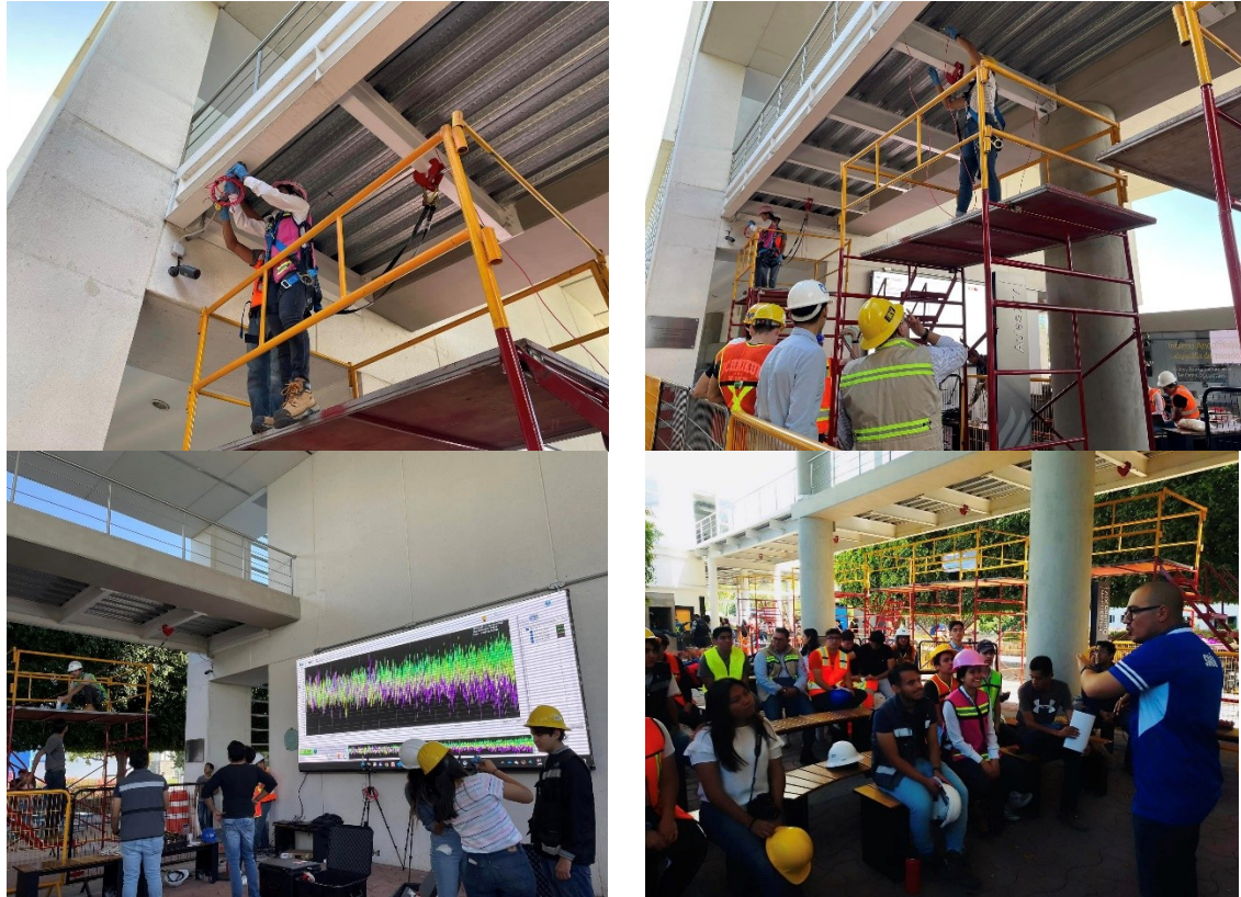
Fig. 11 Instrumentation and loading tests on the bridge
