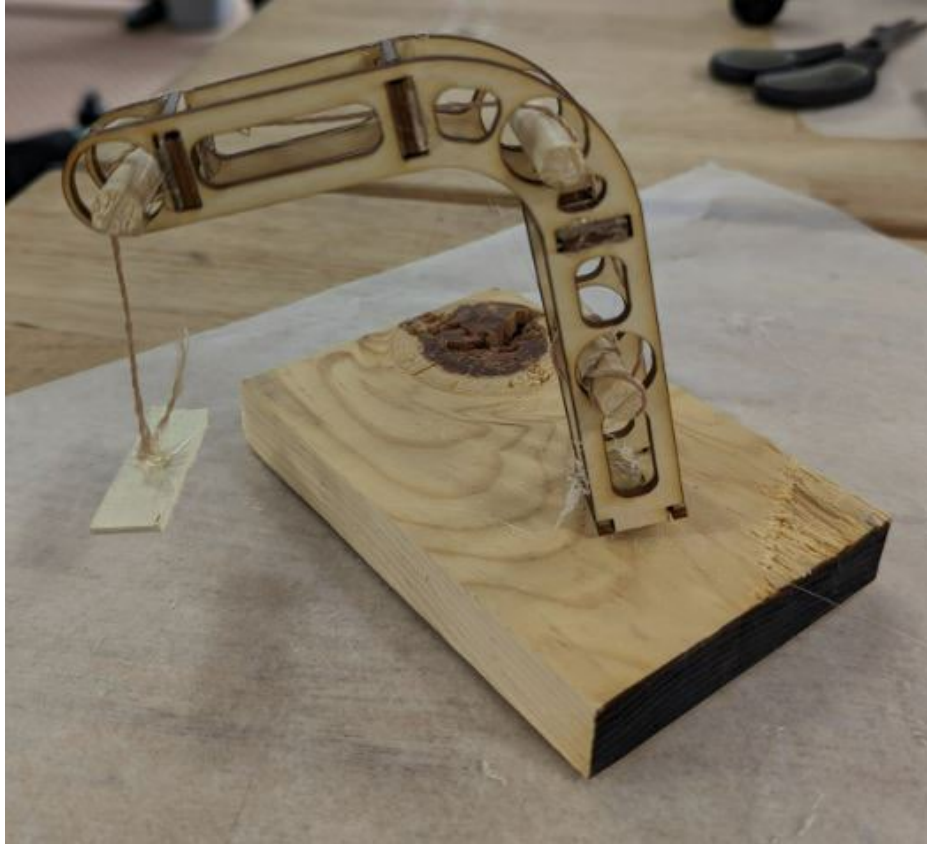
Figure 2: Prototype built by Group C that used a laser engraver to cut a crane device out of wood.
