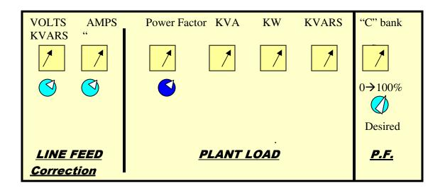
MOTOR LOAD POWER FACTOR CORRECTION SYSTEM USING SOFTWARE THAT WILL CORRECT THE POWER FACTOR TO A DESIRED "SET" VALUE.
