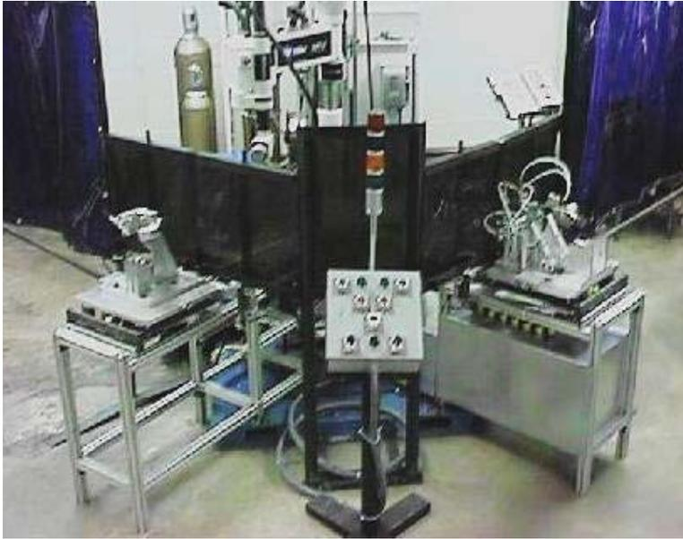
Figure 4. Front View of Actual Automated Welding Cell
