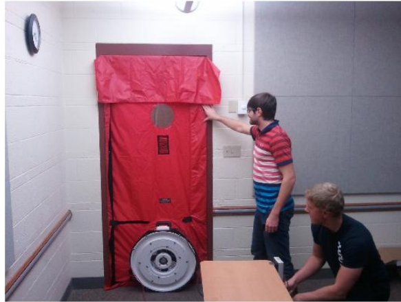
Figure 6: Blower Door apparatus
