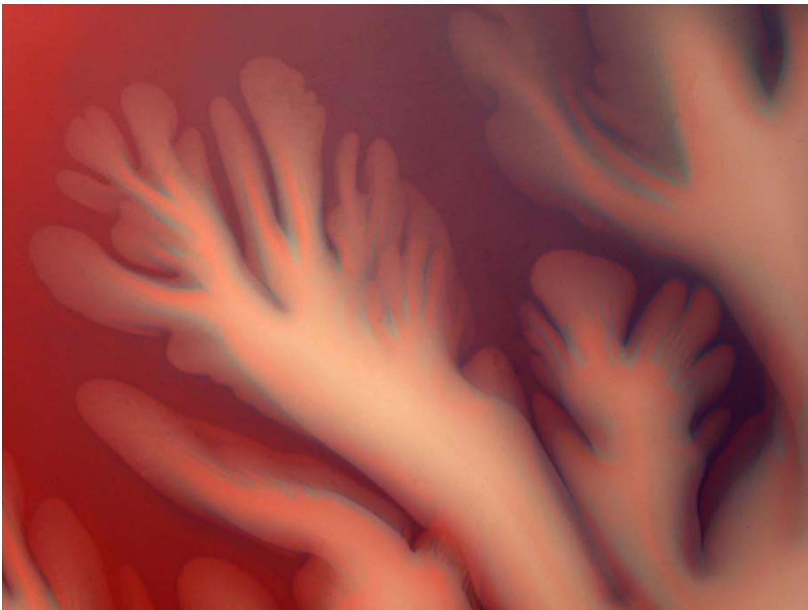
Figure 6: Saffman-Taylor Instability in a Hele Shaw Cell . Marilyn Poon, Jessica Todd, Robert Neilson, Dustin Grace.
