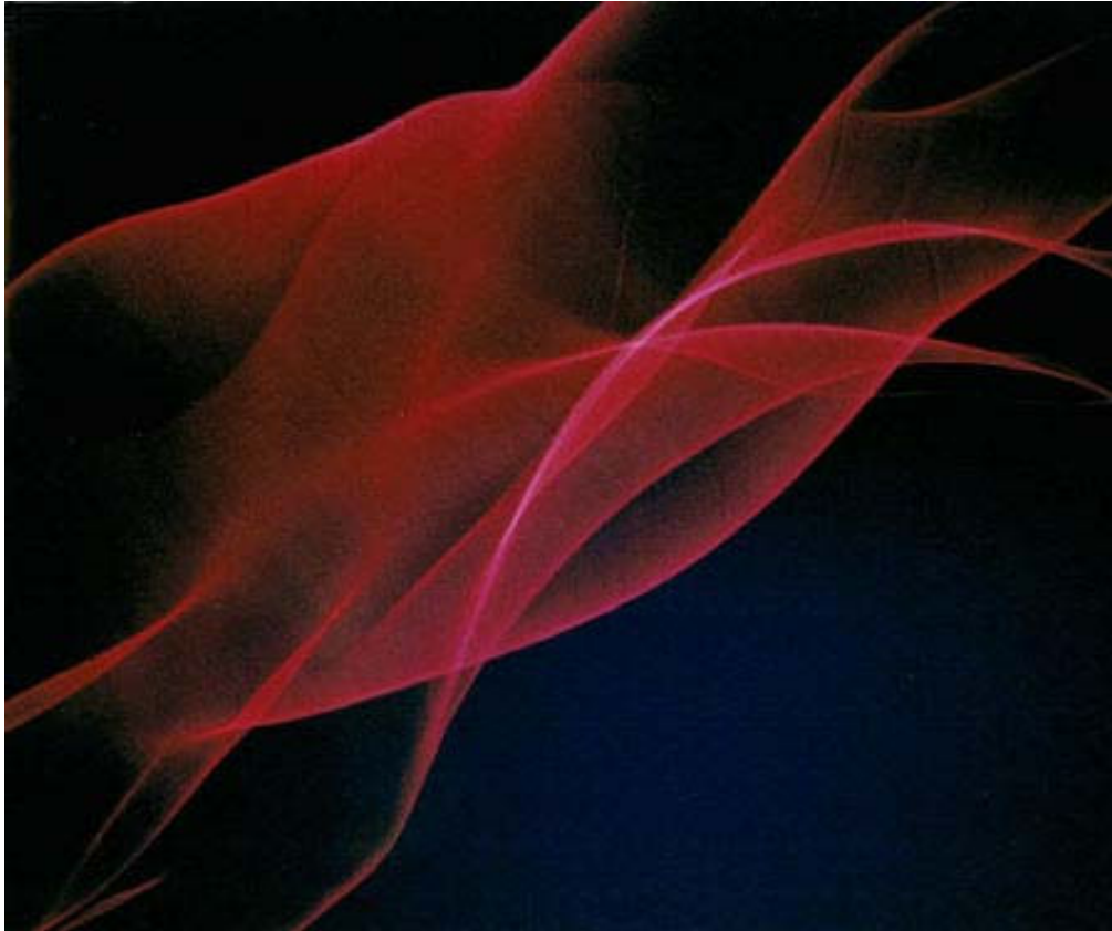
Figure 5: String in Turbulence . A timed exposure reveals the motion of three 1.5 mm diameter strings in the turbulent flow generated by a box fan.
