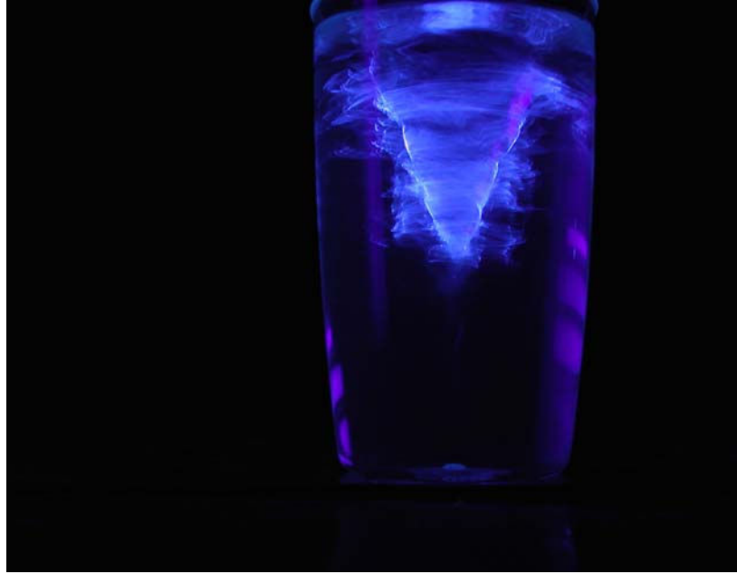
Figure 2: All Vortex . A vortex was formed manually, using an egg beater in a circular cylinder. A fluorescent marker (All laundry detergent) was added from above and excited by UV light. Geoffrey Hill.
