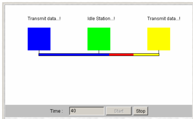
Figure 5: Two stations transmitting simultaneously leading to collision
