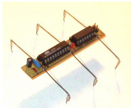
Figure 8: SMA driven robotic bug
