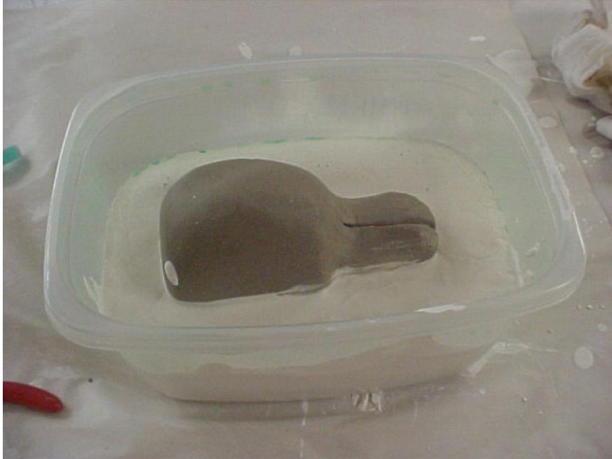
Figure 3: Using earth clay patterns in making plaster molds
