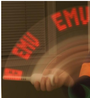
Fig. 4 A Persistence of Vision Wand with its image display.
