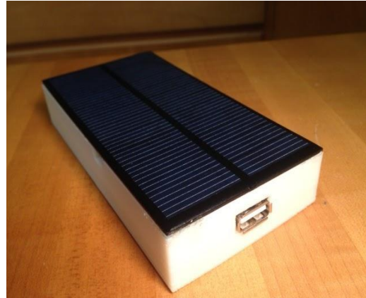
Fig. 3 An assembled solar-powered cell phone charger developed by students in the course.
