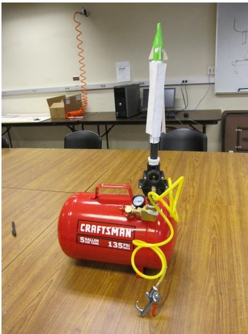
Figure 1 Compressed-Air Launcher Apparatus
