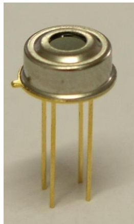
Figure 11. MLX90614 Infrared sensor in a TO-39 container.
