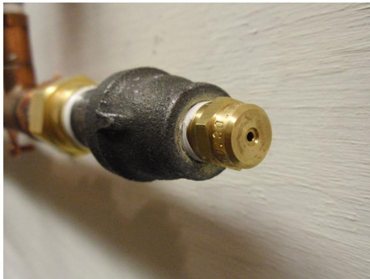
**Figure 5 - Manufactured Nozzle Mounted on Experiment**
