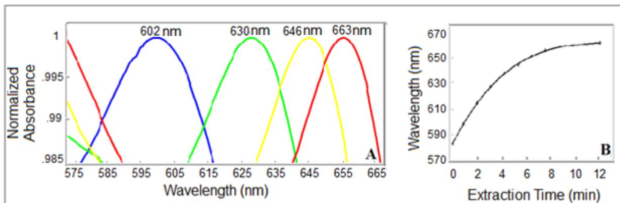
**Figure 2:** (A) Normalized absorbance spectra for CdTe quantum dots extracted from the reaction vessel at 1, 3, 5 and 11 min which yield absorbance maxima of 602, 630, 646 and 663 nm, respectively. (B) The absorbance maxima of the quantum dots versus the extraction time from the reaction vessel.
