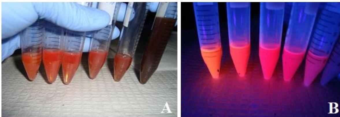
**Figure 1:** Images showing solutions containing CdTe quantum dots illuminated with (A) visible and (B) ultraviolet light. The extraction times, from left to right, are 0.5, 1, 1.5, 2, 2.5, 3 and 3.5 min, respectively.
