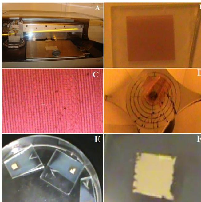
**Figure 4:** Optical images of (A) the Dimatix Materials Printer DMP-2800 used for Printing CdTe quantum dot ink, (B) the substrate after the ink has been printed, (c) the ink after annealing, (D) spin coating of the cell with the PEDOT:PSS polymer, (E) the final cell and (F) the top gold contact.
