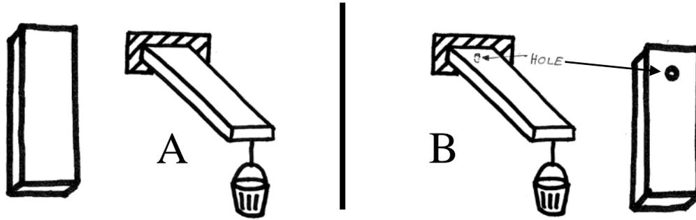
Two beams made of a ductile metal are cantilevered to a wall. The beams are identical except that beam B has a small hole drilled in it as shown. Load is slowly applied to each beam by filling the bucket attached to each beam with sand. Both buckets are filled at the same rate. Which of the following best describes the expected results of the experiment?
