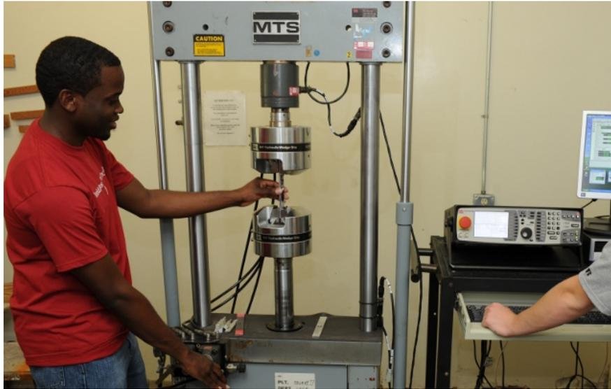
Figure 3: Installation of fatigue test specimen in servohydraulic testing machine
