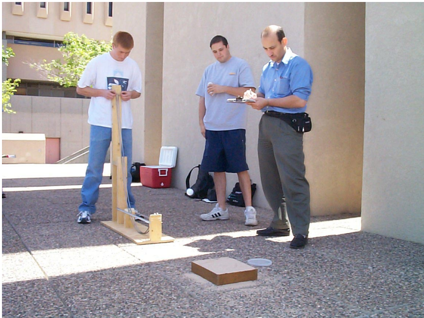
Figure 2. Another slide design that released a golf ball from a certain height off the ground to gain linear momentum.
