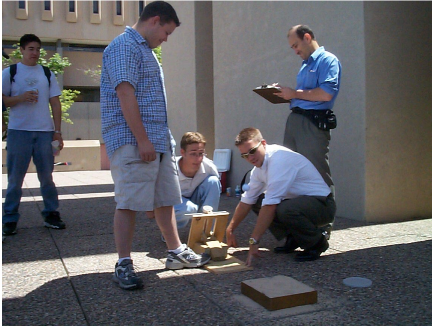
Figure 3. A design utilizing a compression spring tilted at an angle from the floor.
