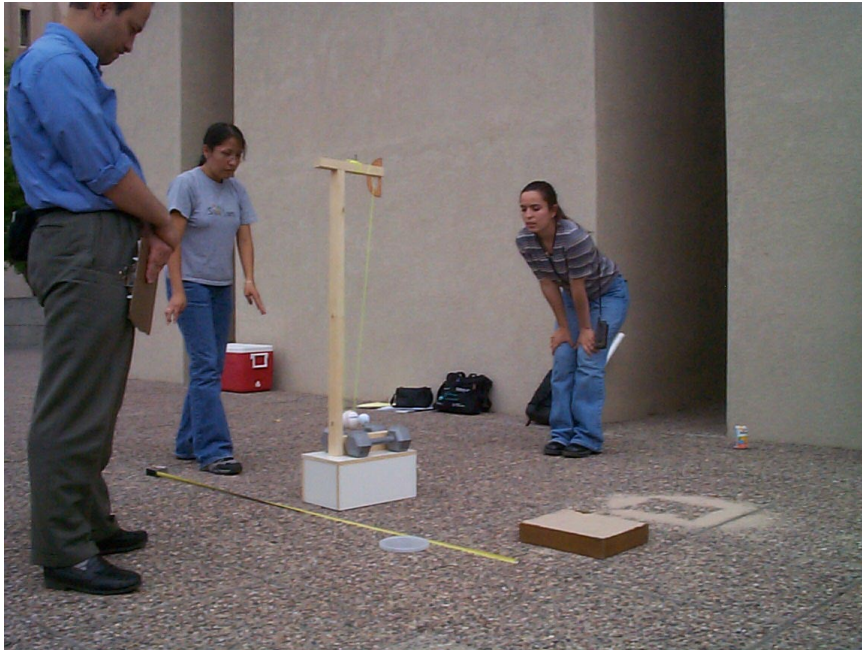
Figure 5. A design that relied on the impact of a pendulum with the golf ball in order to shoot the ball in the air. In this picture, the pendulum (composed of a baseball attached to strings) is showing as it was just about to hit the golf ball.
