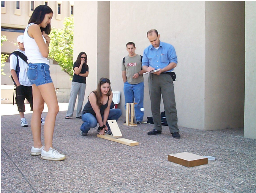
Figure 4. A torsional spring design where the ball rested loosely in a smaller hole in a springing wood board.
