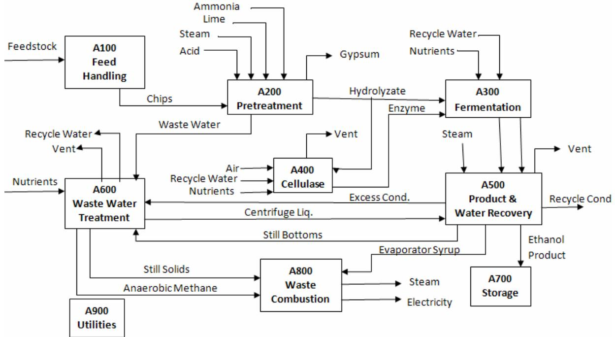
Figure 1. NREL Cellulosic Biomass-to-Ethanol Process (Adaptation)<sup>2,3</sup>
