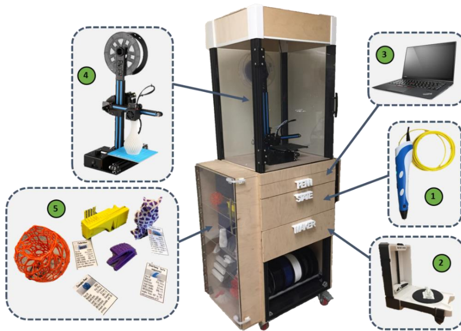
Figure 1. Final "Nittany Build Box" with Supporting Units (1. Extrusion, 2. Scanning, 3. Print Preparation, 4. Printing, and 5. Showcase)
