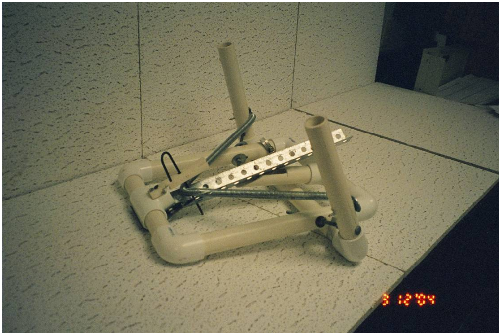
Figure 9: External Extension Spring; Adjustable Tilt
