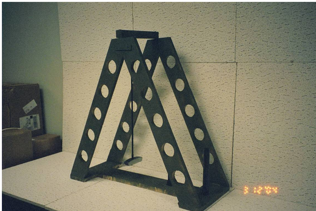
Figure 5: Pendulum Design: Tee Height Adjusted by Replacement
