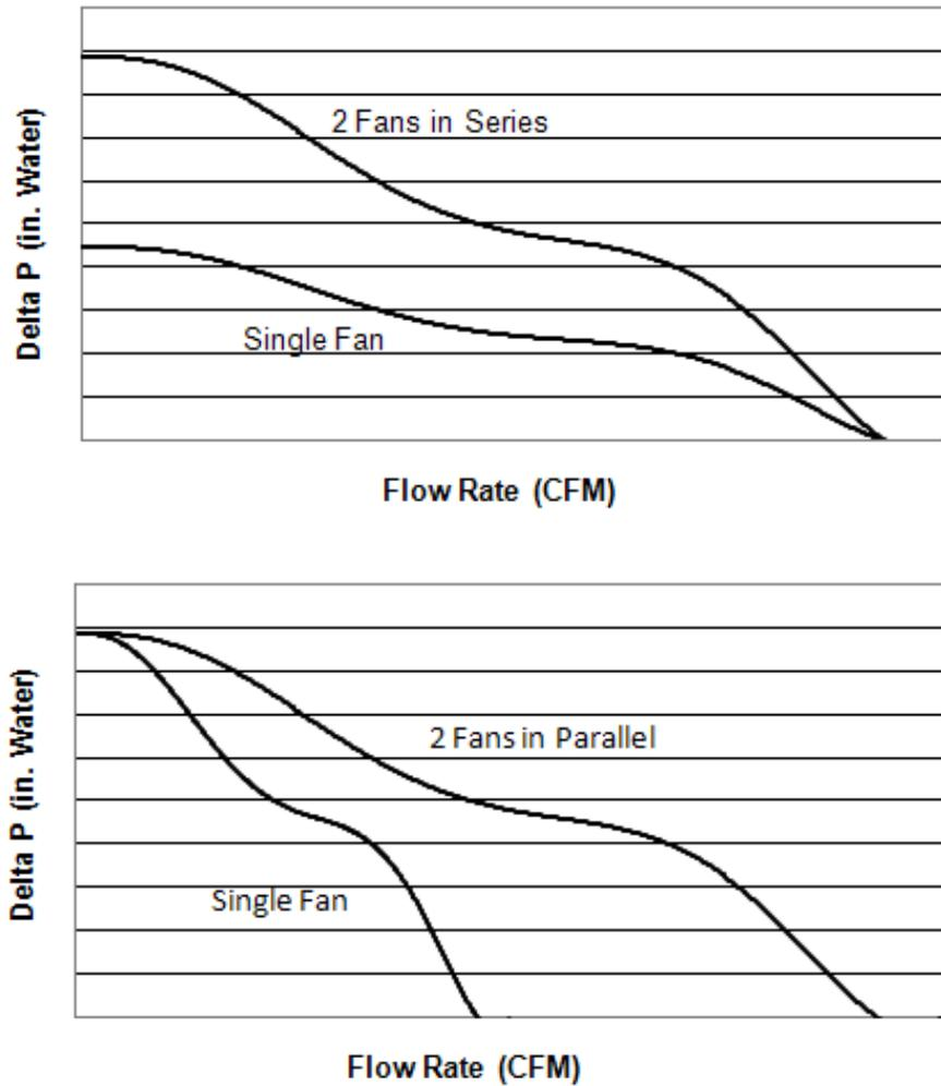
**Figure 8 – Fans in Series and Parallel**
