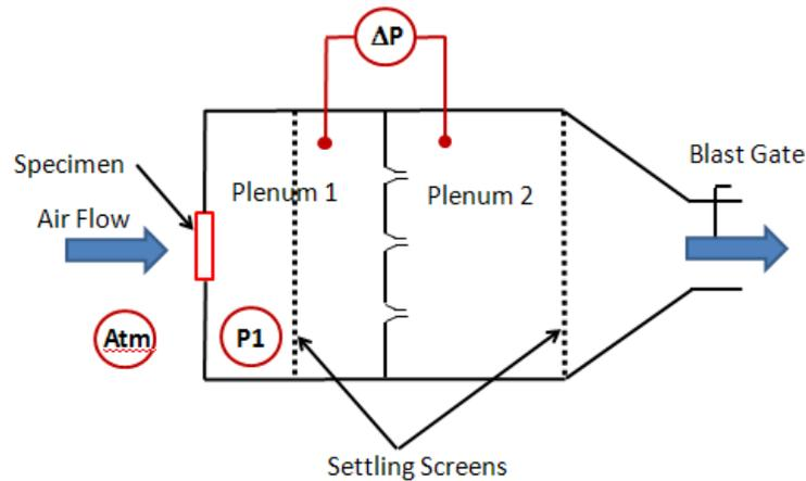
Figure 6 – Schematic of Air Flow Bench
