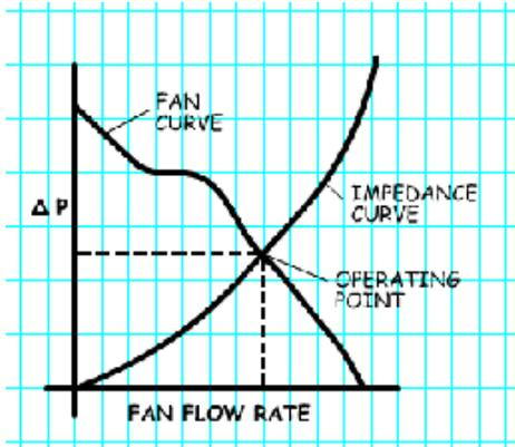
Figure 1 – Operating Point of a Fan
