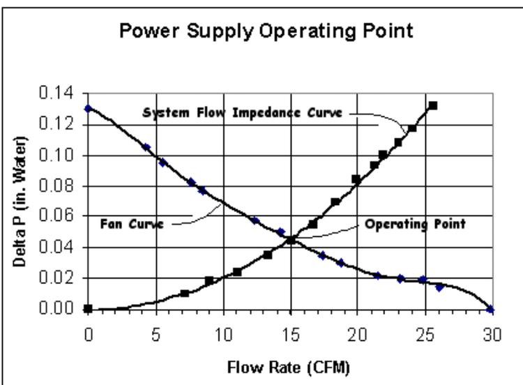
Figure 7 – Plot to Determine Fan Operating Point
