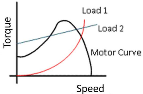
Figure 2 – Operating Point of a Motor
