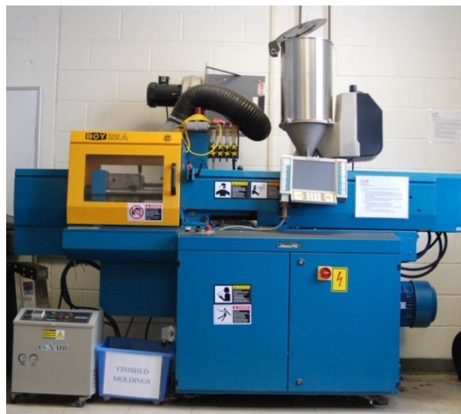
Figure 5. Plastic injection machine
