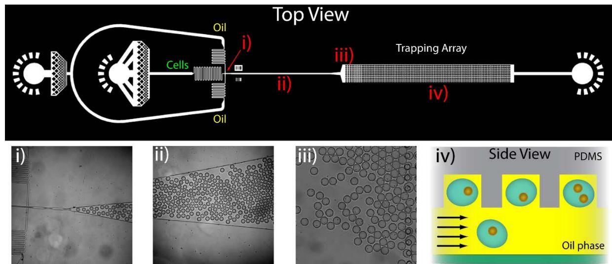
**Figure 3. Overview of the droplet microfluidic trapping array.** (i)-(ii) Generation of monodisperse aqueous droplets containing single cancer cells. (iii) Trapping of aqueous droplets in an array fabricated on top of the microfluidic channel in the PDMS. (iv) Cartoon schematic of the droplet trapping observed from the side.
