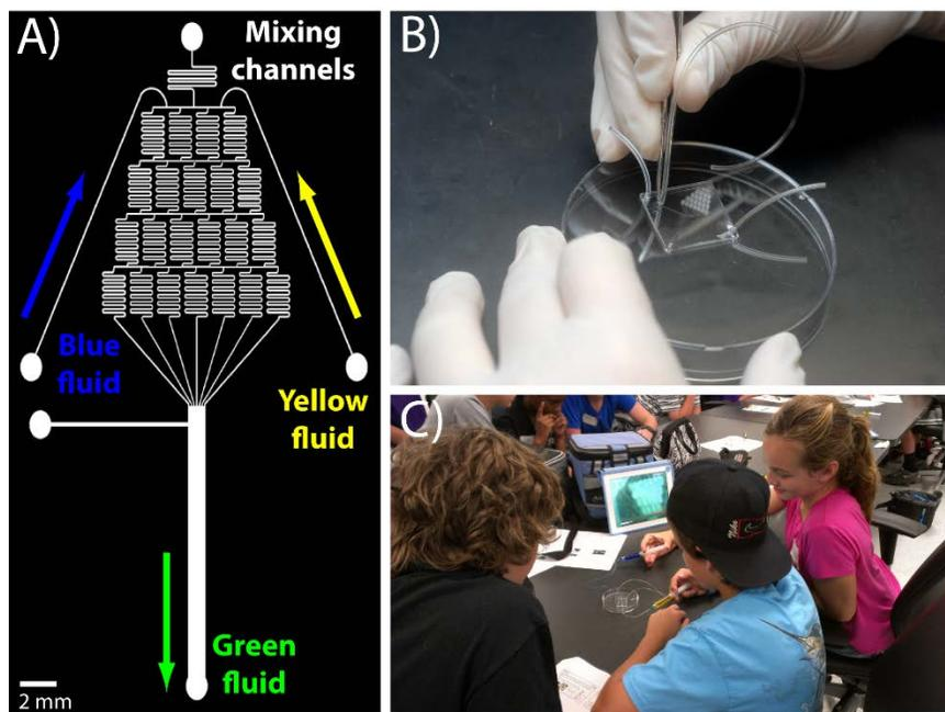
**Figure 1. Design, fabrication, and use of a microfluidic gradient generator.** (A) Schematic of the serpentine gradient generator used in the microfluidics 101 demo that used the device to mix blue and yellow fluids to produce a green fluid. (B) Image of the assembled and plumbed microfluidic device. (C) Students from one of the COE summer camps using the microfluidic device.
