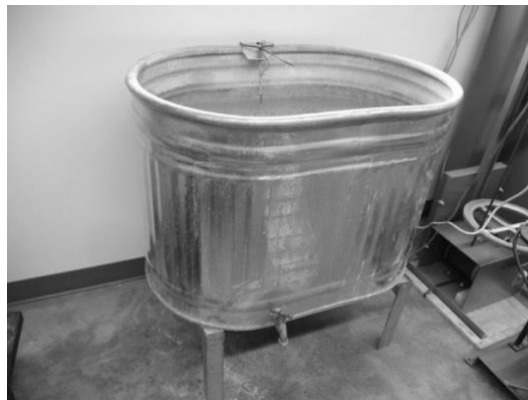
Figure 2. Concrete cylinder curing tank
