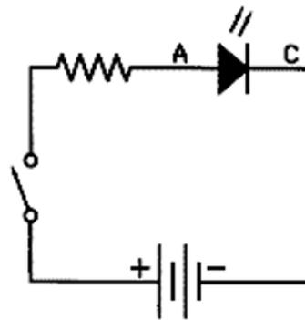
Figure 2: LED Circuit
