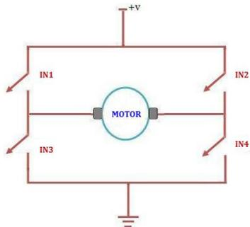
Figure 6: H-Bridge schematic
