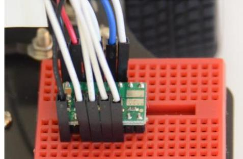
Figure 7: H-Bridge with wiring
