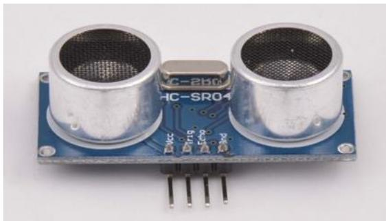
Figure 10: HC-SR04 Ultrasonic sensor
