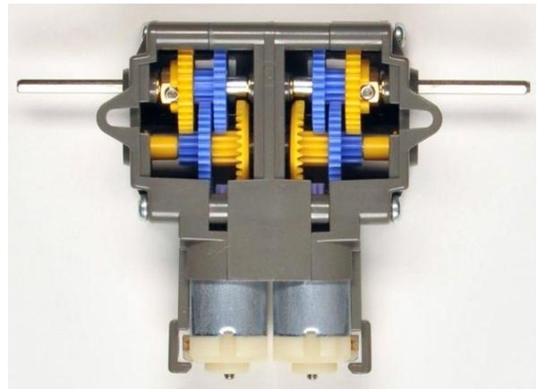
Figure 4: Assembled gearbox
