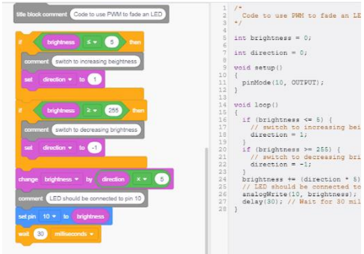
Figure 3: Tinkercad has both text coding (right) and code blocks (left). When using code blocks, Tinkercad also creates the text version.
