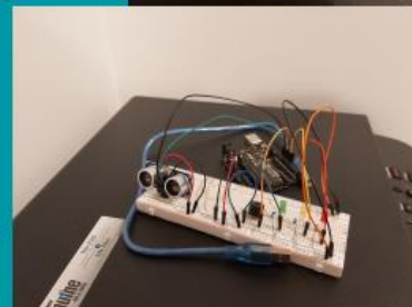
Figure 2: Use of both Tinkercad and a real Arduino for an ultrasonic sensor project.
