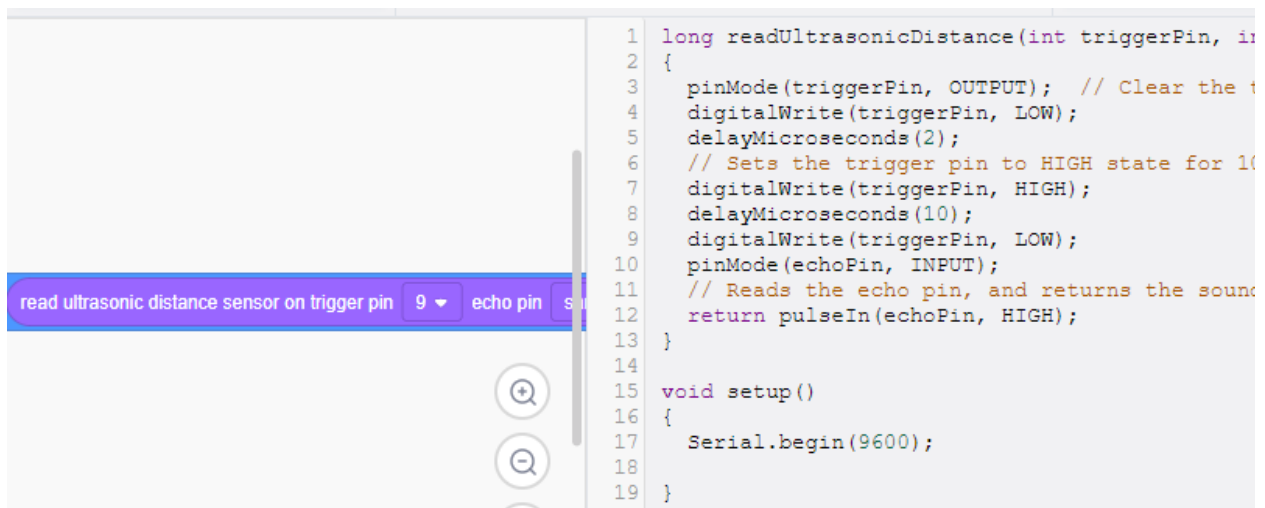
Figure 4: The ultrasonic sensor code block is an example of how all the text coding required by the Arduino is automatically created by Tinkercad Codeblocks.
