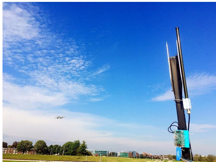
Figure 10. Close-up photo of deployed ADS-B Receiver.
