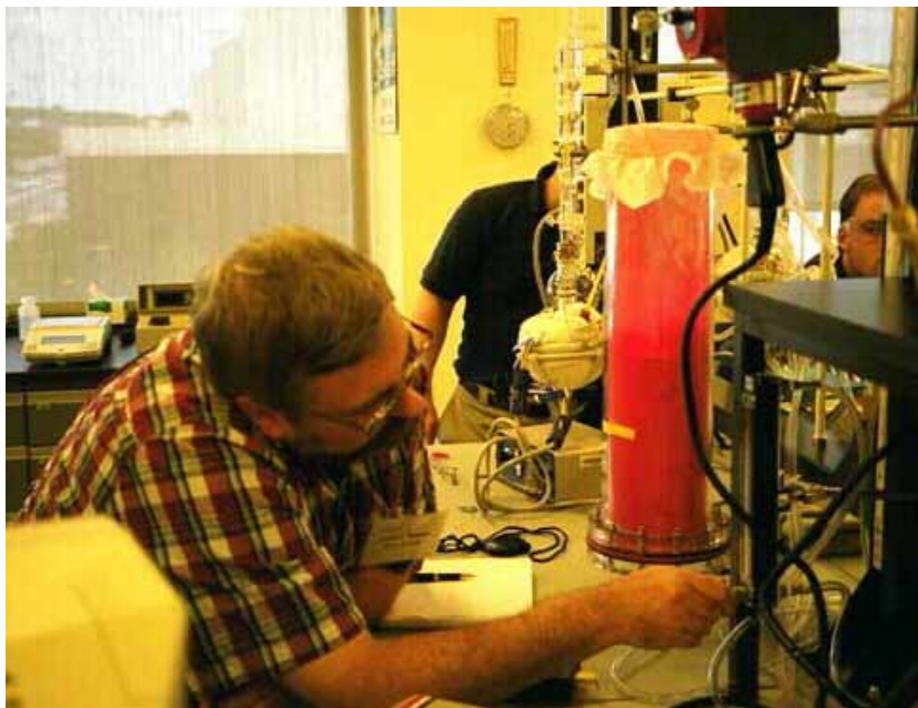
1999 NSF Faculty Workshop Participants Doing Fluidized Bed Polymer Coating Experiment
