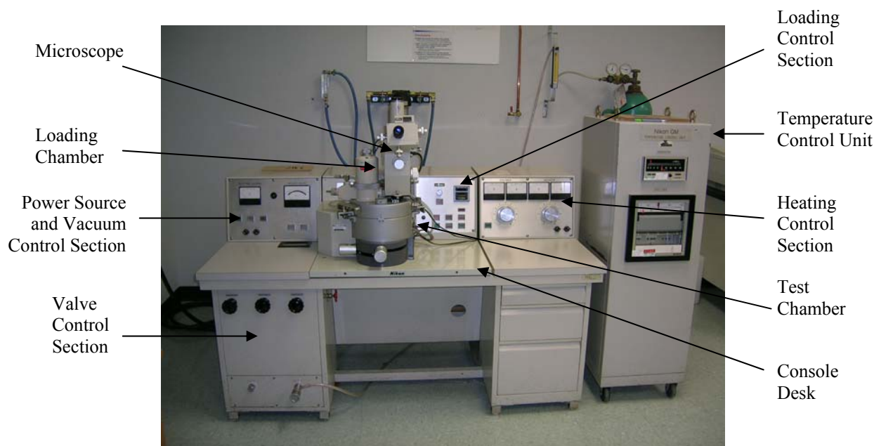
Fig. 3: Nikon QM Hot Microhardness Tester at the Surface Engineering Laboratory, University of Arkansas
