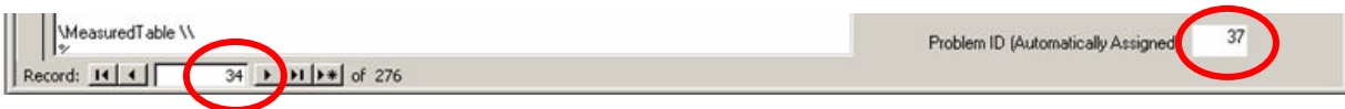
Figure 6 – Problem ID and record number for a particular problem. Note that the record number (34) differs from the Problem ID (37) because previous problems were deleted.
