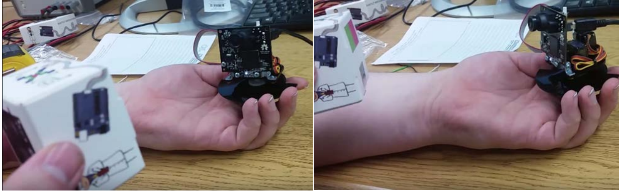
Figure 4: The Pixy camera sends out a signal to its servos in order to keep the box in the center of its field-of-view.
