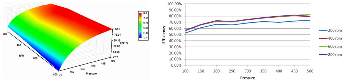
Figure 2. Efficiency mapping of an axial piston pump.
