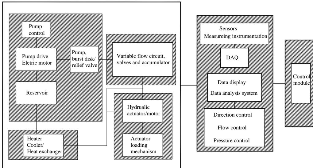
Figure 4. Layout of fluid power system laboratory.
