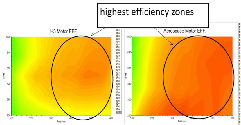
Figure 3. Efficiency mapping of a hydraulic motor.
