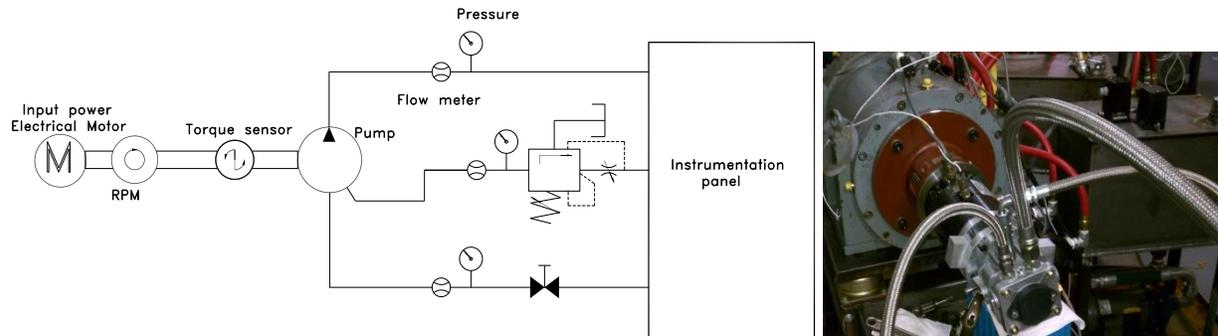
Figure 1. Instrumentation for efficiency mapping test cell.
