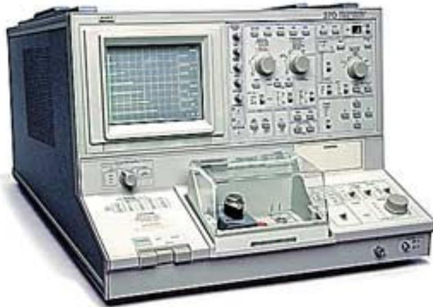
**Figure 1:** Tektronix 370 Curve Tracer
