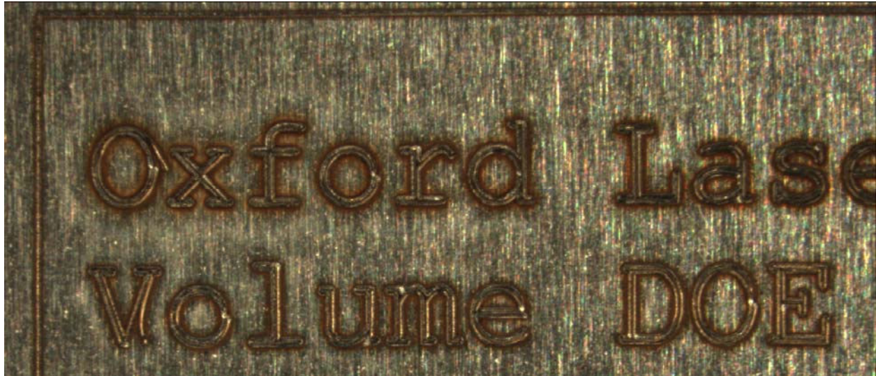
Figure 2: 301 stainless steel machined on Oxford Laser
