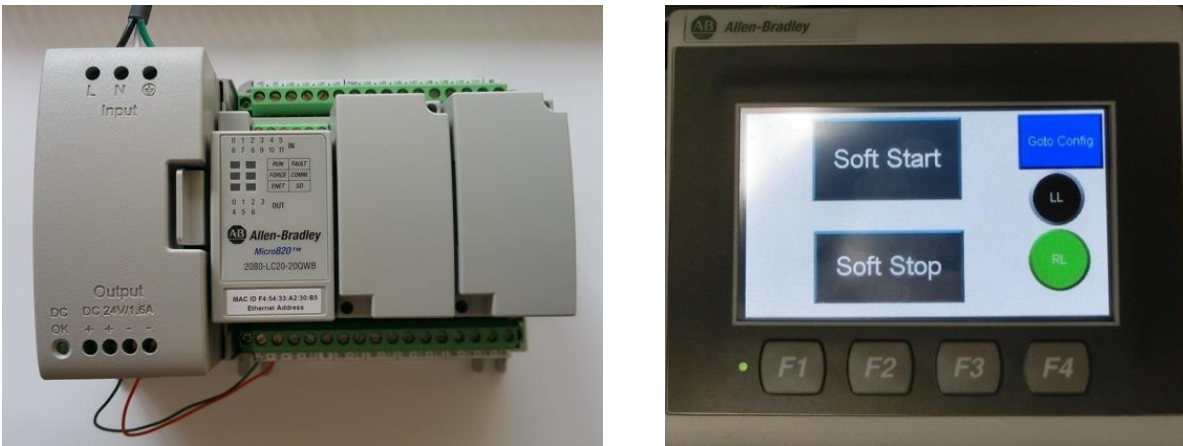
(a) (b) Figure 3. (a) AB Micro820 PLC (b) HMI PanelView800 Terminal
