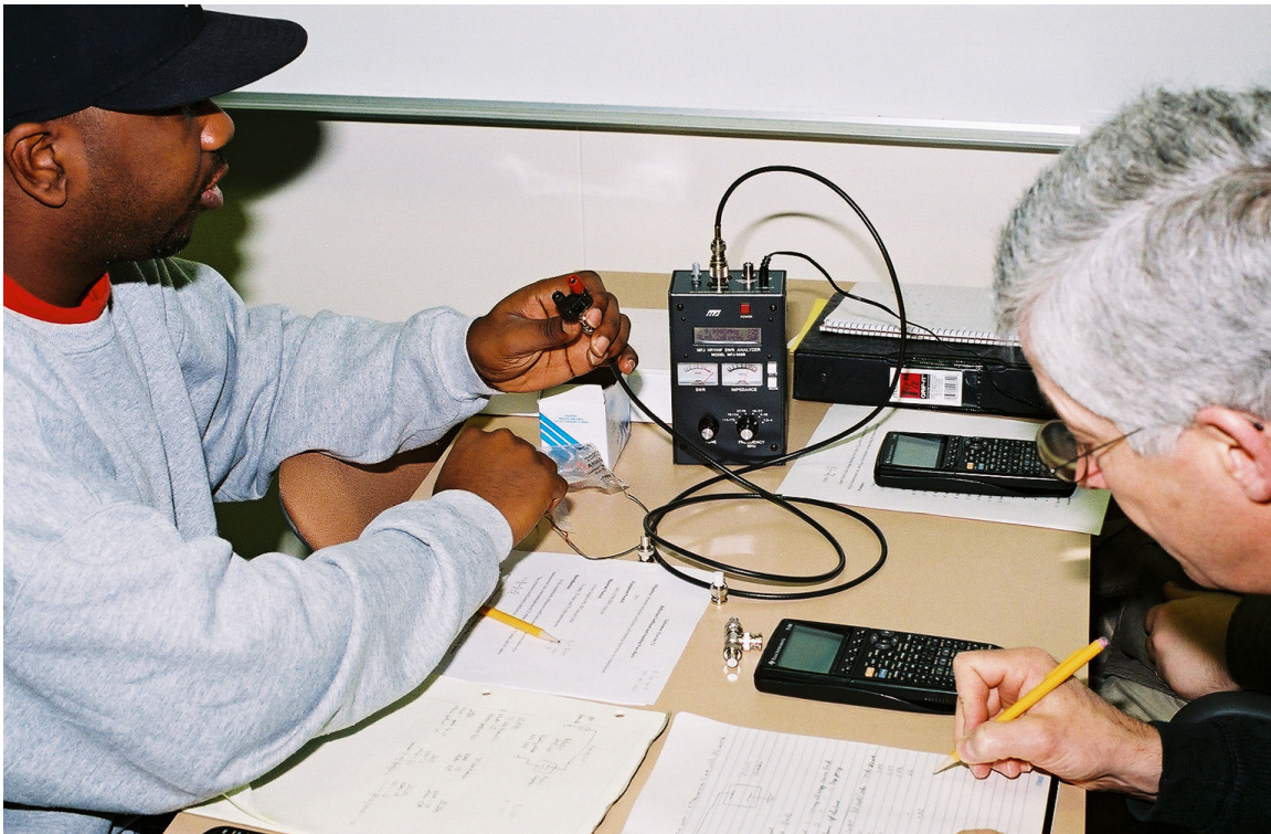
Figure 1. Students performing transmission line laboratory exercises using the MFJ-259B SWR Analyzer.
