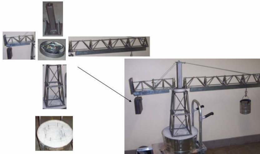
Figure 4. Roof panel lift mechanism
