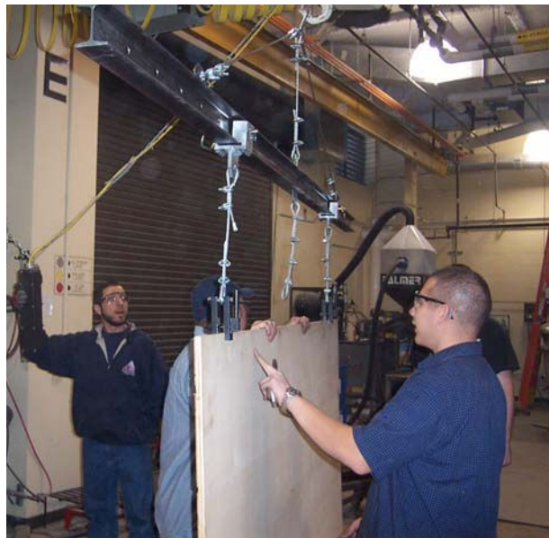
Figure 2. OSB placement mechanism
