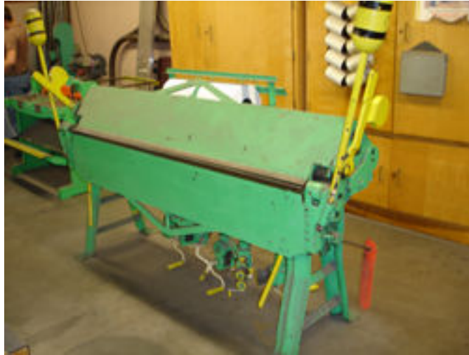
Figure 3. Sheet metal bending machine used for bending book covers
