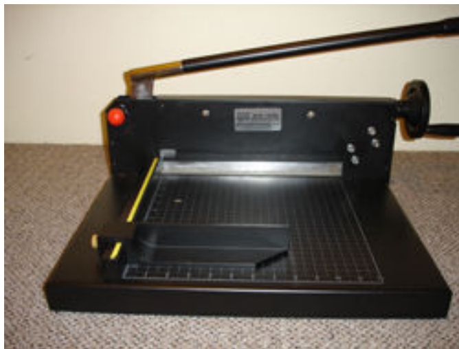
Figure 4. QCM-1200E desktop paper cutter with a paper clamp
