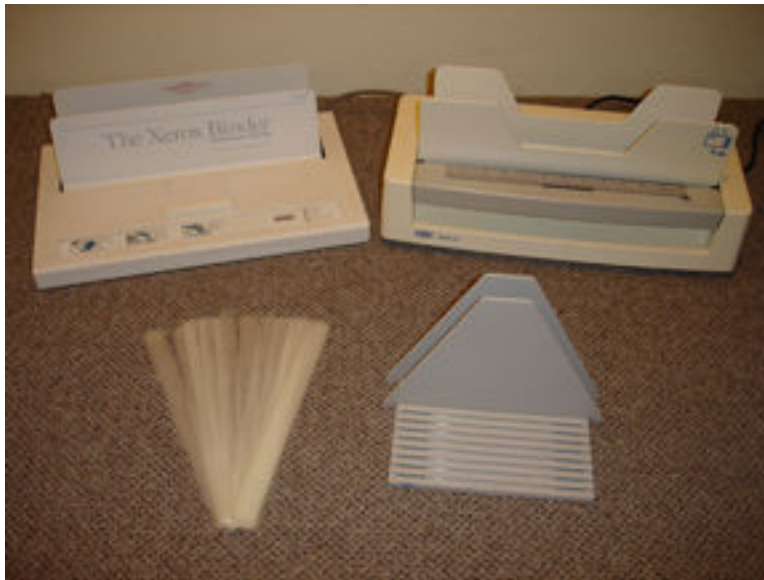
Figure 5. Binders with a cooling rack and thermal glue strips
