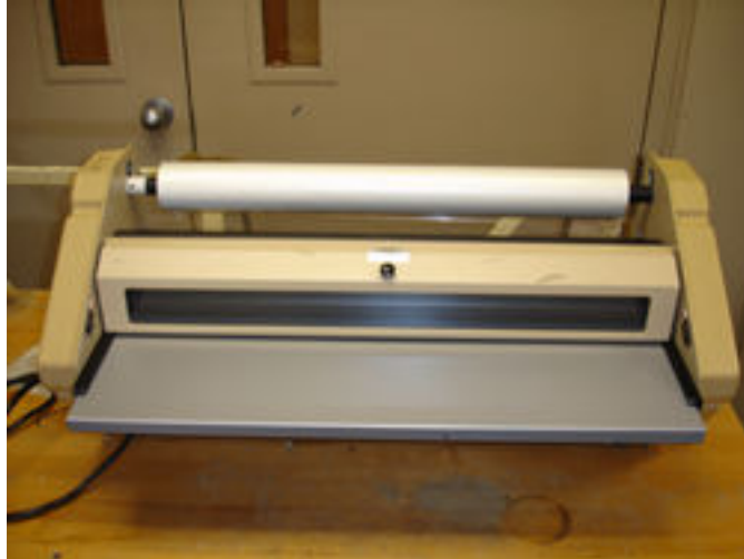
Figure 1. EZ27 roll laminator used in the book-making laboratory
