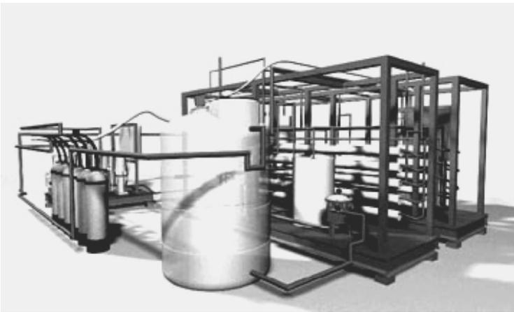
**Figure 6.** Modeled RO water system.
