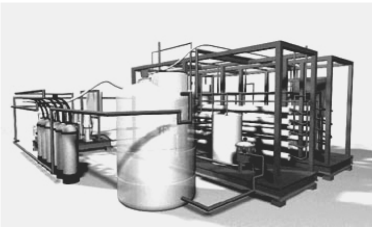
Figure 6. Modeled RO water system.
