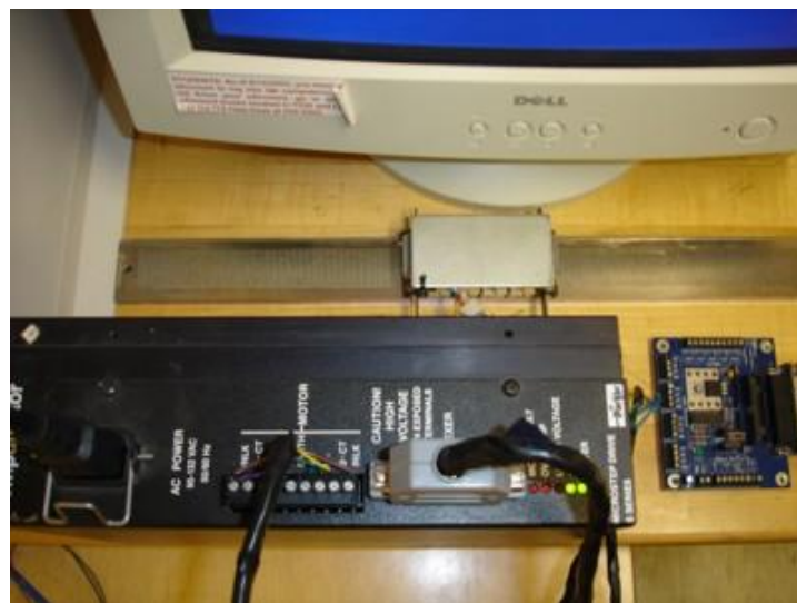
Figure 2. Linear Stepper Motor Forcer on a Track Connected to a Microstepping Drive and a Parallel Port Interface
