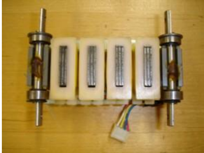
Figure 7. Linear Stepper Motor: Forcer (Bottom View) with Four Windings (in the middle), Two Permanent Magnets (around the shafts), and Four Bearings
