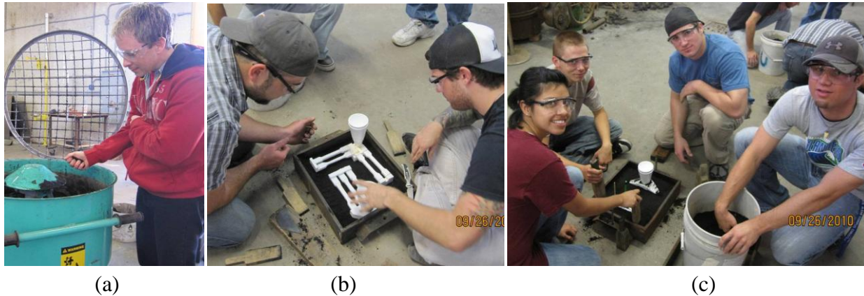
Figure 6: Mixing green sand (a), and compacting it around the patterns inside metal flasks (b) and (c).
