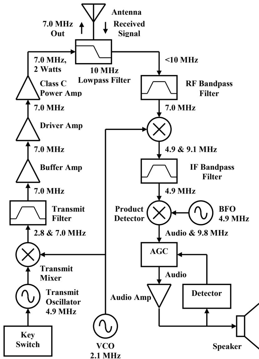
Fig. 1. Block diagram of the NorCal 40A transceiver.
