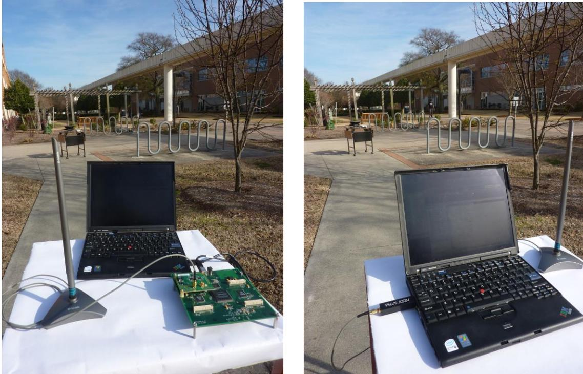
**Figure 9.** Outdoor transmitter-receiver set-ups for the mobile platform
