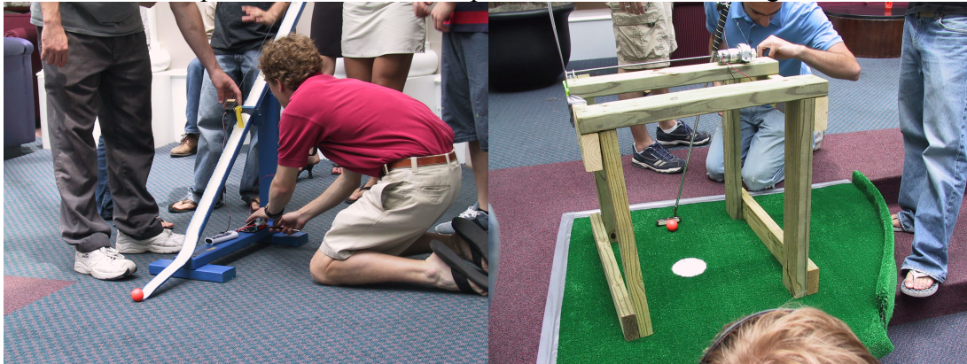
Figure 2. A ramp and a putter style golf robot using DSP control for height and backswing timing, respectively.
