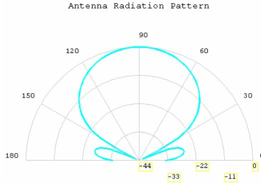
Figure 2: The polar plot of the far-field radiation pattern of a Yagi-Uda antenna.
