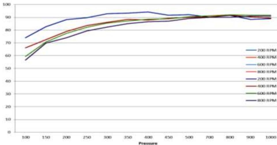
Figure 5 Hydraulic motor overall efficiency versus pressure
