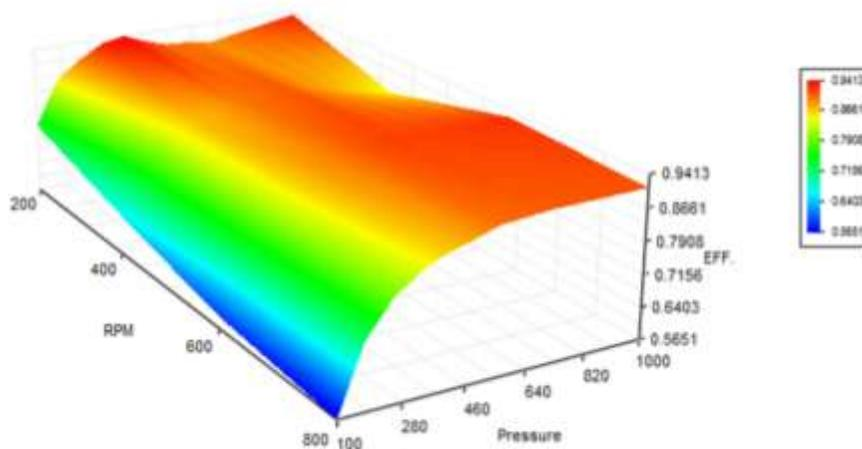
Figure 6. Efficiency mapping of a hydraulic motor
