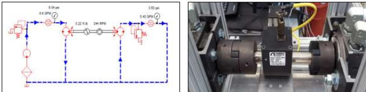
Figure 4. Actuator module and motor-pump coupling
