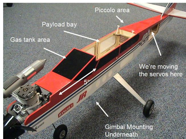
Figure 4 – Hardware Layout<sup>4</sup>
