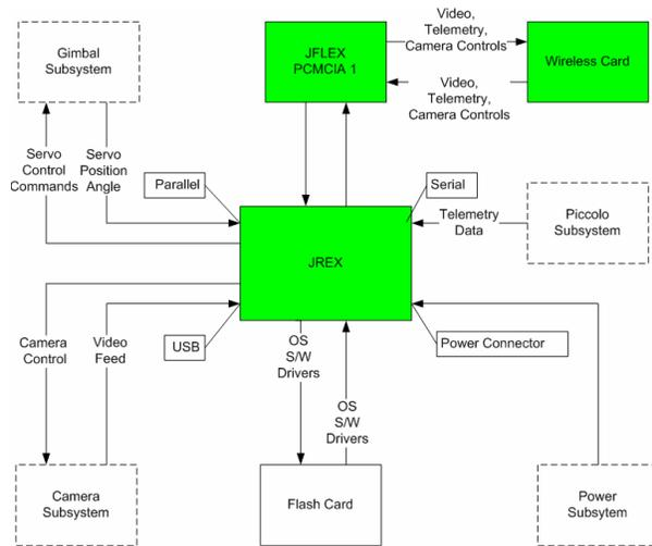
Figure 2 – UAV System Top-Level Block Diagram<sup>4</sup>
